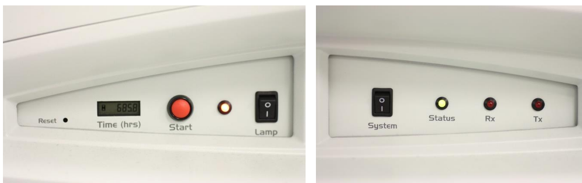
Figure 2.1: The front panel, including lamp panel (left) and system panel (right)
