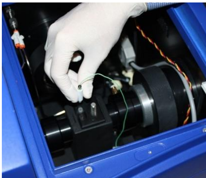
Figure 2.5: Inserting the temperature thermocouple
