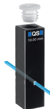
Figure 6. A highly focused beam of 1.5 mm width delivers maximum accuracy.
